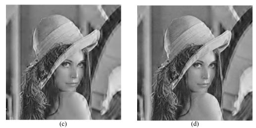
Fig.7 The subjective results of "Lena" image by BER=10e-3, bit rate=1bpp in the lowest  $H_{L_3}$  subband. (a) Reconstructed image by error free, PSNR=36.21dB; (b) Error resilience only by resynchronization marker, PSNR=14.49dB; (c) Missing wavelet coefficients replaced by zeros, PSNR=27.05dB; (d) Reconstructed image by our proposed algorithm, PSNR=29.64dB.
